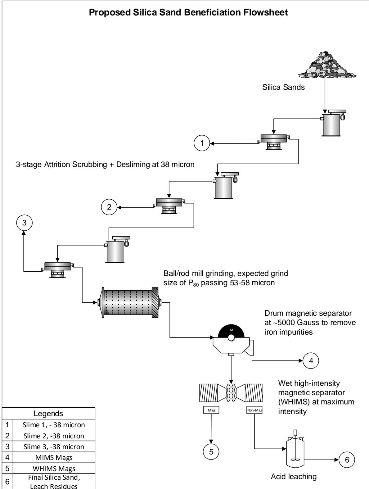
**Figure 9: Proposed Silica Sand Beneficiation Flowsheet (test validation required)**
