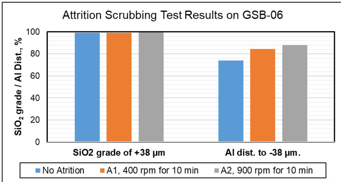
Figure 4: Attrition Scrubbing Test Result Summary on Silica Sand GSB-06 Sample
